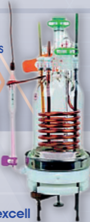
Set-Up for Critical Pitting Temperature Measurements
